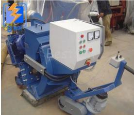
Portable conctere road surface shot blasting machine is a relatively common and common shot blasting machine.
