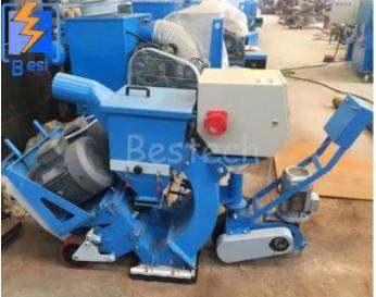
Shot through mechanical method of the pill (steel shot or sand) at high speed and certain Angle to work on the surface of the trajectory, let the pill material impact work, in order to achieve surface shot of surface coarsening and remove residual effect
