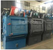
Q32 series crawler shot blasting machine is a small shot blasting cleaning equipment, mainly by the room the shotblast cleaning, shot blasting machine assembly, hoisting machine, separator, shot blasting machine electrical system and other accessories.
