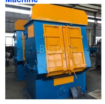
The automatic feeding crawler type shot blasting machine is a shot blasting device with good cleaning effect, compact structure and low noise. It is applied to the surface derusting or shot blasting strengthening of large and medium batch production
