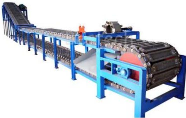
Aluminum alloy fluid into the casting machine of distributor, the distributor uniform injection chain casting machine of aluminium ingot mold, and the ingot mould through spray type cooling make aluminum ingots through sufficient cooling and coagulation.
