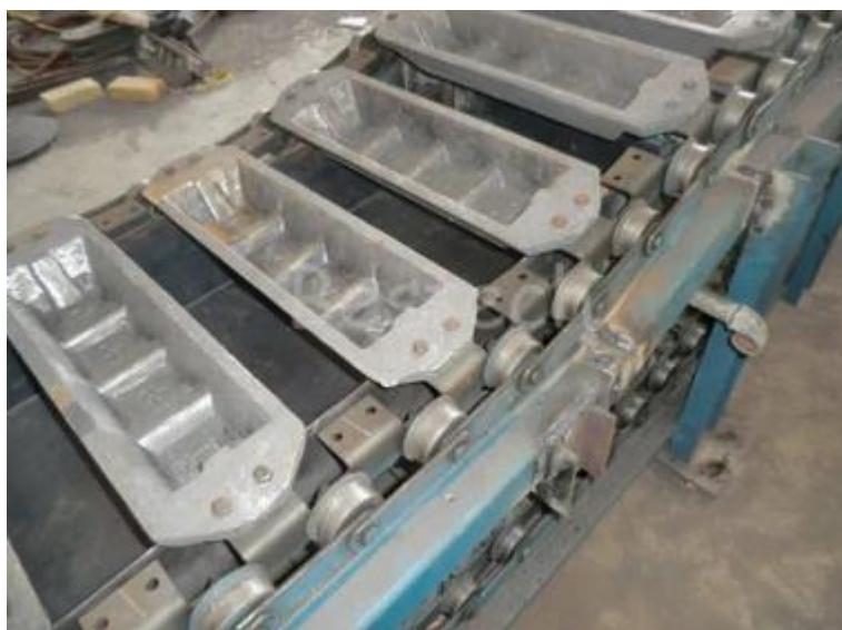
Casting machine mainly include the frame part, drive part, transmission part, mould parts, shunt parts, vibration and cooling part.
