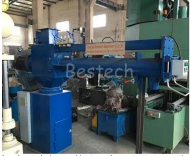
foundry sand mixer machine has a frame structure supporting two half shells, which form the mixing tube. These are split length-ways and are hinged at a single point behind the sand inlet.
