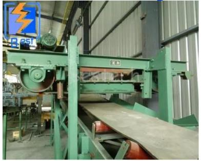
Green sand processing production line is an eddy centrifugal mechanical regeneration device. Sand through quantitative device falls down regeneration plate of high speed rotation
