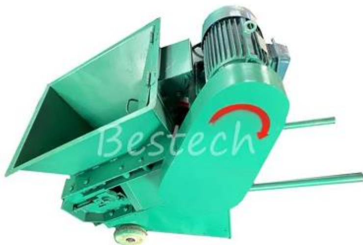
Foundry vibration knockout machine for resin sand and clay sand reclamation line
