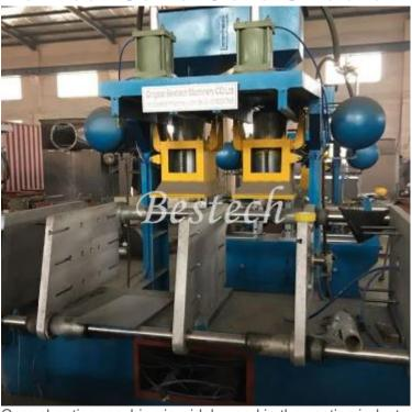
Core shooting machine is widely used in the casting industry. The core shooting machine makes the core with precise size and smooth surface.
