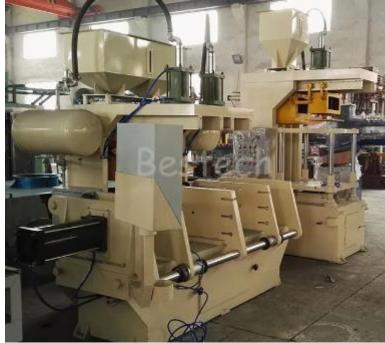
Vertical type shooting sand core molding machine is the most widely used in the foundry industry, and the cores manufactured by the core shooting machine have accurate dimensions and a smooth surface.
