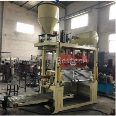
Z6540 cold box(hot box) core shooting machine is vertical parting, and the moving mold can be flipped and put the same core into conveyor belt.
