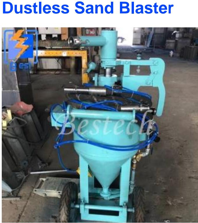
Sandblasting machine is a new kind of surface treatment equipment, widely used in metal rust & welding slag removal, building surface cleaning, wood restoration, coating & paint removing, oil containment removal, road marking line cleaning etc.
