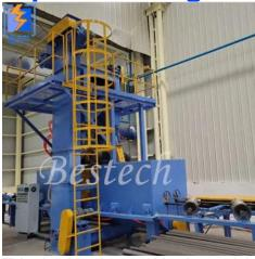
This shot blasting machine is special for cleaning elbow pipe, steel pipe and irregular - shaped tubes and soon on
